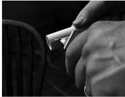
Trimming up the slot with a utility knife
