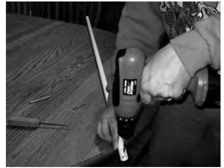
Drilling the 3/16" hole
