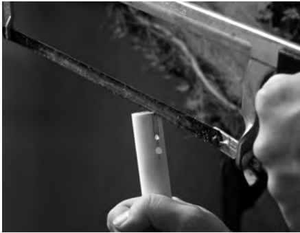
Cutting the slot with a hacksaw
